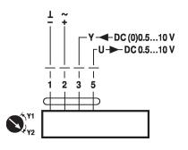
Override control (frost protection circuit)
