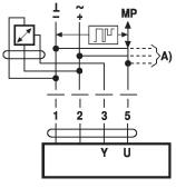
Connection of external switching contact
