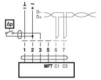
Requirements for switching contact: The switching contact must be able to accurately switch a current of 16 mA @ 24 V.
