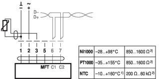
1) depending on type 2) Resolution 1 Ohm Compensation of the measured value is recommended
