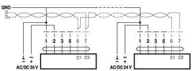
Cable colours: 1= black 2 = red 3 = white 5 = orange 6 = pink7 = grey BACnet / Modbus signal assignment: C1 = D- = A C2 = D+ = B
