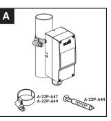
The tightening strap is included in the scope of delivery
