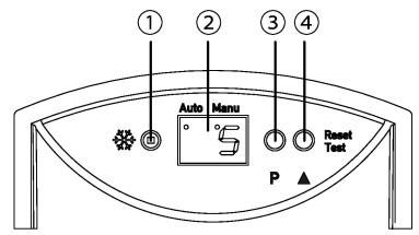
① LED red (danger of frost) ② Display screen for switching point (P) and operating mode ③ Parameter button ④ Value / Reset button
