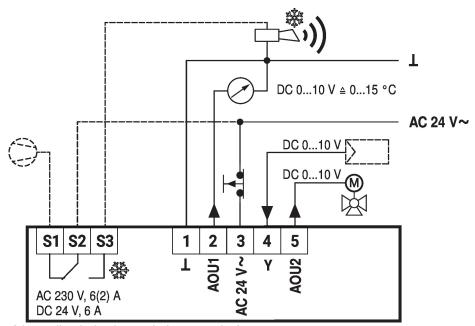
If the capillary leaks, the switch changes to the frost position. Min. active length material of capillary tube is 250 mm. Permissible cable length at 1.5 mm² diameter is max. 300 m.
