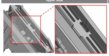
Fix the upper part of the housing on the underside with the screw included in the delivery.
