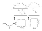
In case of outdoor installation avoid direct rain and sun contact. Probably use sun respectively rain protection. Cable entry from bottom or side. For side cable routing set loop so that precipitation can drain defined. Observe permissible ambient condition.
