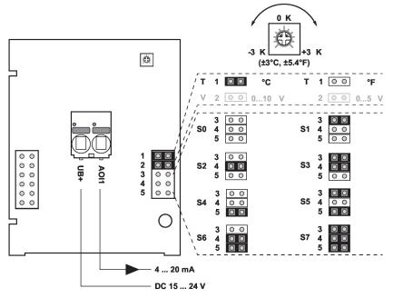
The adjustment of the measuring ranges is made by changing the bonding jumpers. The output value in the new measuring range is available after 2 seconds.
