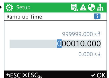
Enter required Ramp-up Time
