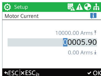
Enter Motor Current from rating label
