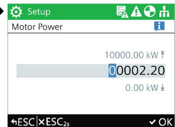
Enter Motor Power from rating label
