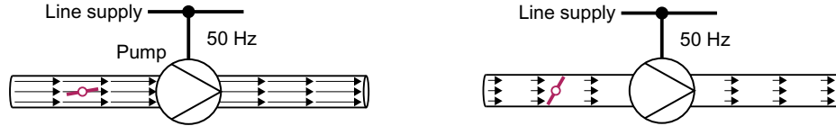
Figure 6-74 Flow control with pump and throttle connected to a 50 Hz line supply
