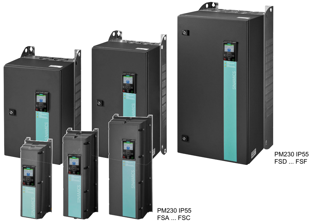
Figure 3-1 PM230, 3-phase 400 VAC, degree of protection IP55 / UL Type 12
