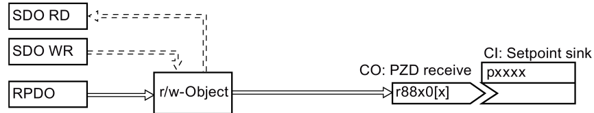
Figure 6-1 Access to mapped PZD setpoint objects
