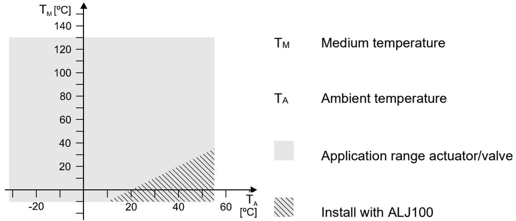
Only use GDB.., GDD..,GSD.. and GQD.. actuators at medium temperatures  $> 0\text{ }^{\circ}\text{C}$ .
