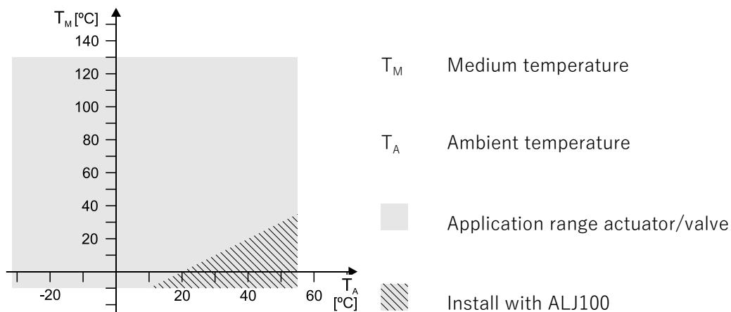
Only use GDB.., GSD.., GQD.. and **GDD.. actuators** at medium temperatures  $> 0^{\circ}\text{ C}$ .
