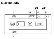
Tool = Configuration and maintenance interface (7-pin)
