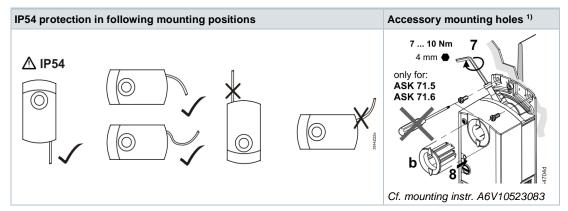
**A** 1) Not to be used for fixation of the actuator, use anti-rotation-bracket instead.
