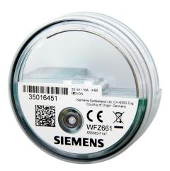
The add-on radio module WFZ661 records and processes the counting pulses of mechanical water meters prepared for wireless transmission and transmits the data to a readout system. It can be configured via an optical interface.
