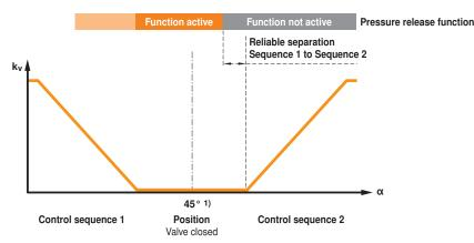
Positioning signal for closed position:
