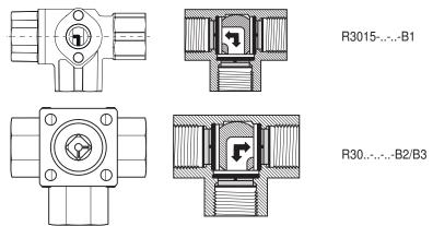
Delivery condition conforms to valve position 90°/positioning signal 10 V.
