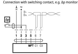
Modbus RTU / BACnet MS/TP with analogue setpoint (hybrid mode)
