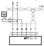
Requirements switching contact: The switching contact must be able to accurately switch a current of 16 mA@24 V.
