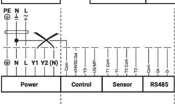
Power supply must not be connected to the signal terminals!
