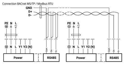
Connection BACnet MS/TP / Modbus RTU with analog setpoint (hybrid mode)
