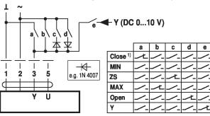
Override control and limiting with AC 24 V with rotary switch
