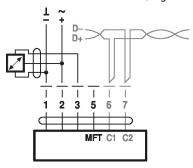
Connection with switching contact, e.g. Δp monitor
