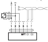
Connection with switching contact, e.g. Δp monitor
