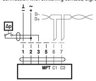
Modbus RTU / BACnet MS/TP with analogue setpoint (hybrid mode)
