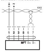
Signal assignment KNX: D+ = KNX+ (pink > red) D- = KNX- (grey > black) The connection to the KNX line should take place via WAGO connecting terminals 222/221.
