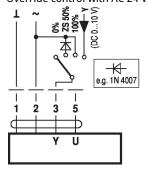
Control remotely 0...100% with positioner SG..
