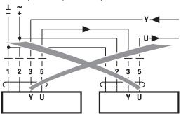
Control with 4...20 mA via external resistor
