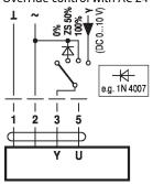
Control remotely 0...100% with positioner SG..
