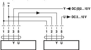
Control with 4...20 mA via external resistor
