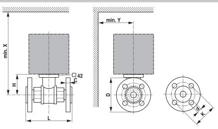
X/Y: Minimum distance with respect to the valve centre. The actuator dimensions can be found on the respective actuator data sheet.
