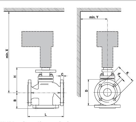
X/Y: Minimum distance with respect to the valve centre.
