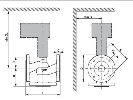
X/Y: Minimum distance with respect to the valve centre.
