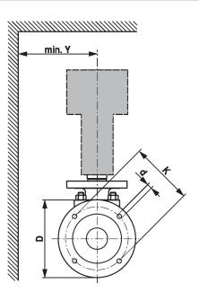
X/Y: Minimum distance with respect to the valve centre.
