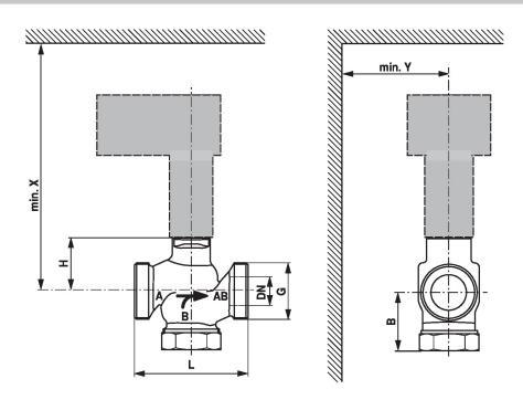
X/Y: Minimum distance with respect to the valve centre.
