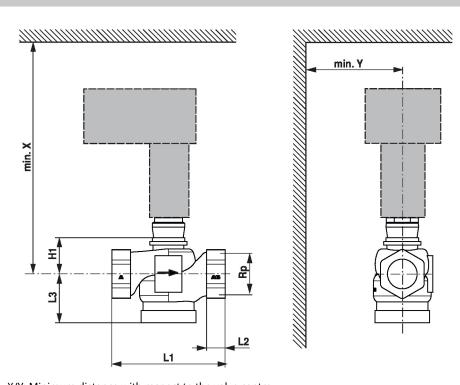
X/Y: Minimum distance with respect to the valve centre.
