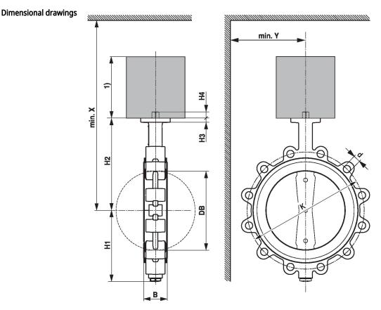
The actuator dimensions can be found on the respective actuator data sheet.
