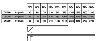
Parametrisation linear characteristic curve
