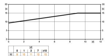
[d] = Electricity interruption in days[s] = Pre-charging time in secondsPF[s] = Bridging time
