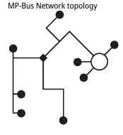
network topology (star, ring, tree or mixed forms are permitted). Supply and communication in one and the same 3-wire cable • no shielding or twisting necessary • no terminating resistors required
