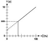
Control with 4...20 mA via external resistor
