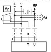
There are no restrictions for the network topology (star, ring, tree or mixed forms are permitted). Supply and communication in one and the same 3-wire cable • no shielding or twisting necessary • no terminating resistors required
