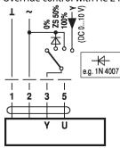
Control remotely 0...100% with positioner SG..
