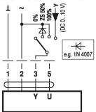
Control remotely 0...100% with positioner SG..
