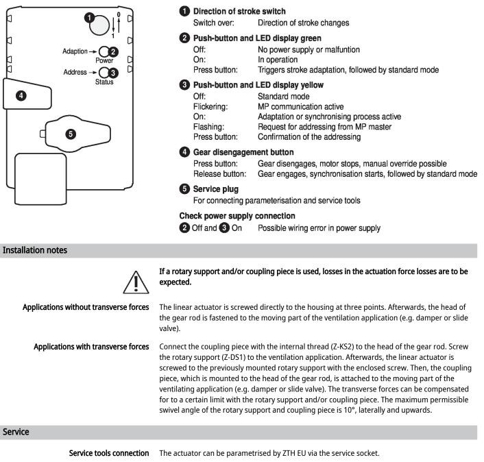
For an extended parametrisation the PC tool can be connected.
