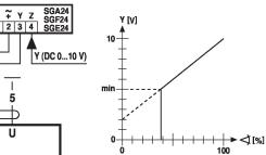
Control with 4...20 mA via external resistor
