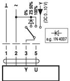
Control remotely 0...100% with positioner SG..
