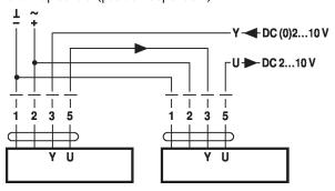
Control with 4...20 mA via external resistor
