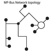
There are no restrictions for the network topology (star, ring, tree or mixed forms are permitted). Supply and communication in one and the same 3-wire cable • no shielding or twisting
