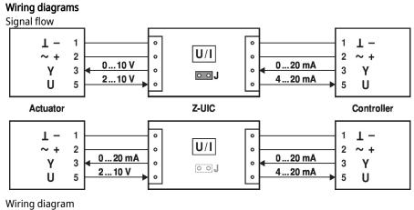
with jumper for actuators SR-,
